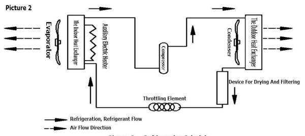
Picture 2 Refrigeration Principle
